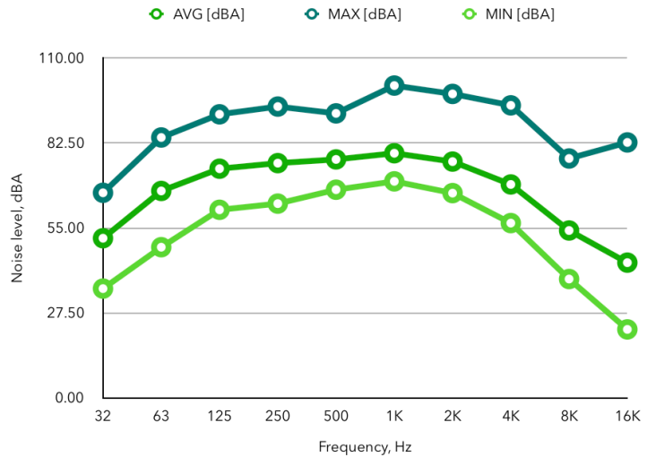
Fig. 9 – table and graph of measurements in a middle-upper class residential area
