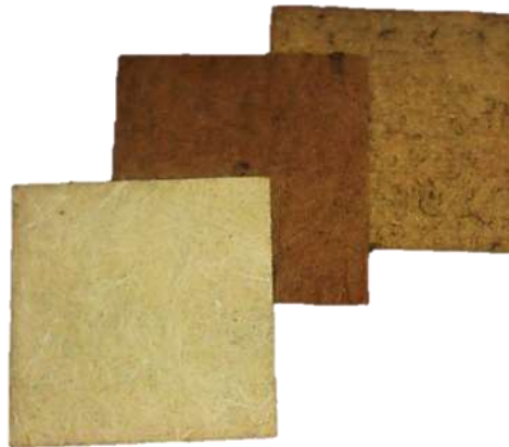
Figure 4. Manufactured samples (upstream): non-woven sample of fique, sample of non-woven and sample in which both types of fibers, fique and coconut are combined.
