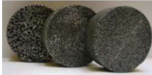
Figure 2. Picture of the aluminium sponges fabricated by the infiltration process.
