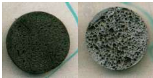
Figure 1. Aluminum foams of approximately 1 and 2 mm average pore size manufactured by the powder metallurgical technique
