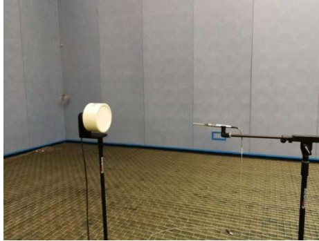
Figure.2 Resonant PZT transducer and the SPL measurement in anechoic room
