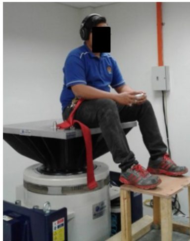
Fig. 3. Experiment set-up with human subject giving response to noise and vibration delivered through headphone and vibration shaker with static footrest.
