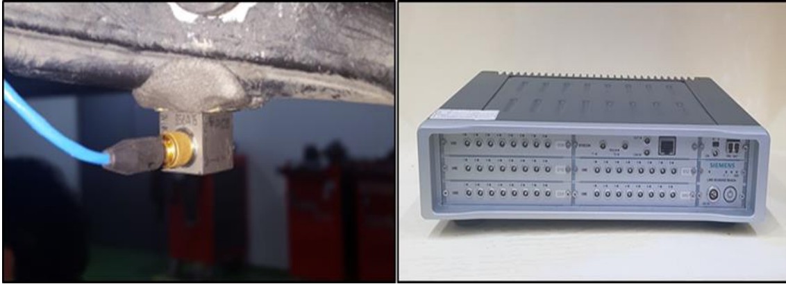
Figure 1. Equipment for vibration signal acquisition: tri-axial piezoelectric accelerometer (right) and LMS SCADAS Mobile (left)
