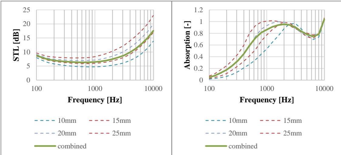
Figure 6: Results for FOAM + EPOXY FELT; STL (left), Absorption (right).
