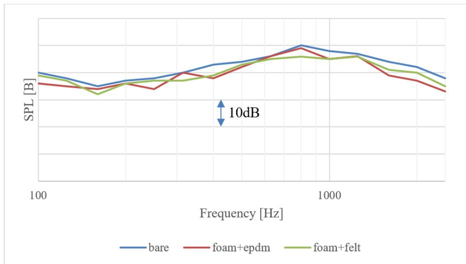
Figure 14: Transfer function from motor to driver head
