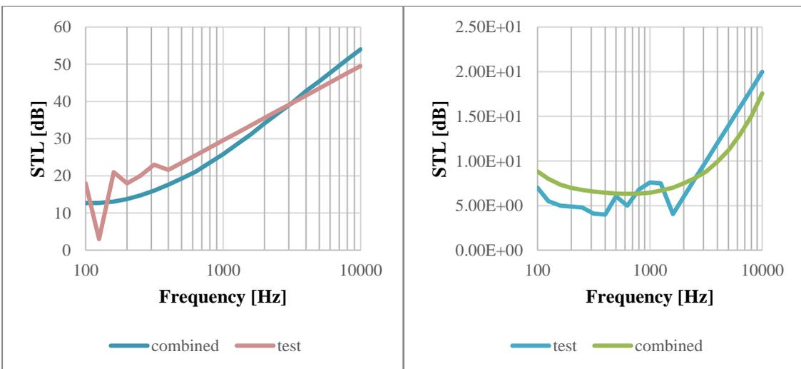
Figure 7: STL comparison. Foam + EPDM (left) and Foam + Felt (right)
