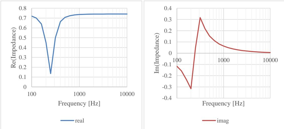
Figure 11: Real and imaginary part of acoustic impedance. Foam + EPDM.
