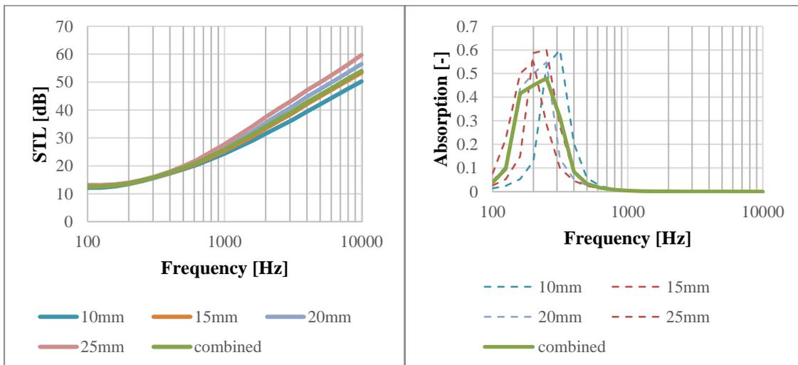
Figure 5: Results for FOAM + EPDM; STL (left), Absorption (right).
