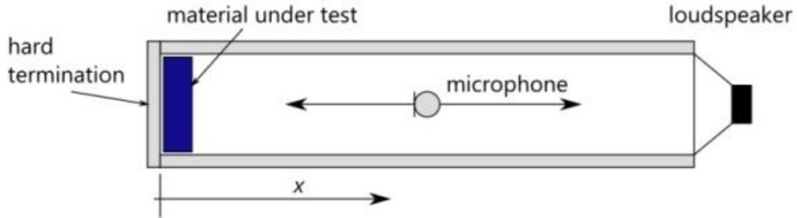
Figure 8: Kundt tube set-up for absorption measurements
