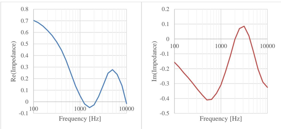
Figure 12: Real and imaginary part acoustic impedance. Foam + Felt.
