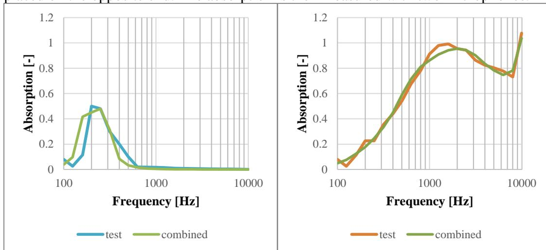
Figure 9: Absorption comparison. Foam + EPDM (left) and Foam + Felt (right)
