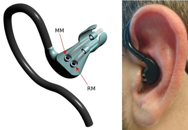
Figure 9: Illustration of the dosimetric earpiece. Left panel: 3D model showing the earpiece, instrumented with a measurement microphone (MM) and a reference microphone (RM). The distance between the tips of the two probe-microphones is 8~mm. The RM's location is intended for measurements near the ECE. The earpiece was designed to allow a maximum insertion depth of approximately 8~mm. Right panel: picture showing the earpiece worn in the ear.
