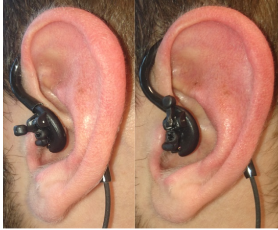
Figure 11: Dosimetric earplug, as worn with the vent in open (left) or sealed (right) conditions.
