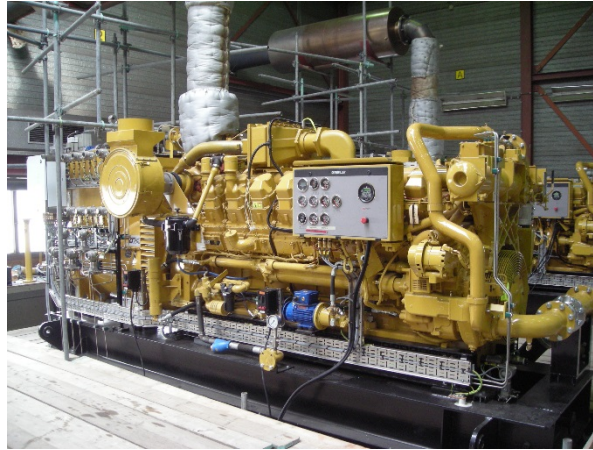
Figure 4: Gas engine during sound power determination
