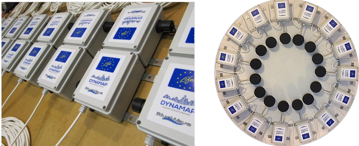
Figure 3. The high computation capacity sensors built for the pilot area of Rome and Milan.
