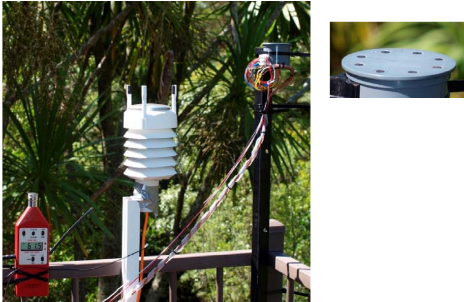
Figure 5. Preliminary field trial setup, showing SPL meter (left), Vaisala weather station (centre), and array arrangement III (right). Also shown at top right is the view of the array from slightly above.
