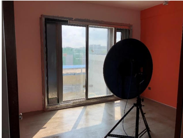
Figure 3 The Acoustic Camera Measurement Setup in the Test Room
