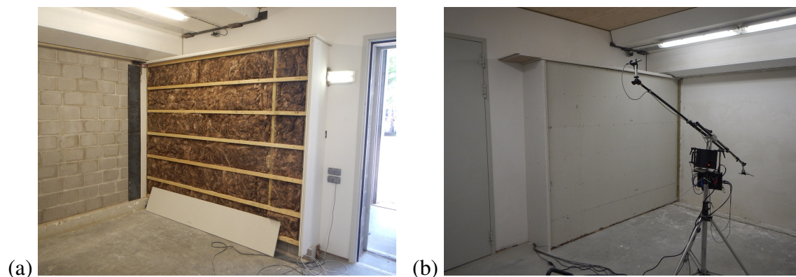
Figure 1: (a) façade test element without interior finishing in the sending room and (b) façade test element with interior finishing in the receiving room.
