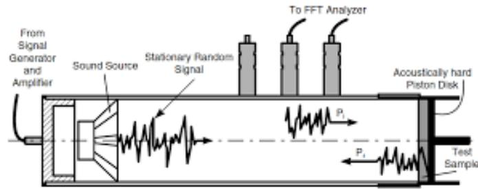
Figure 3. Impedance tube two microphone configuration section view
