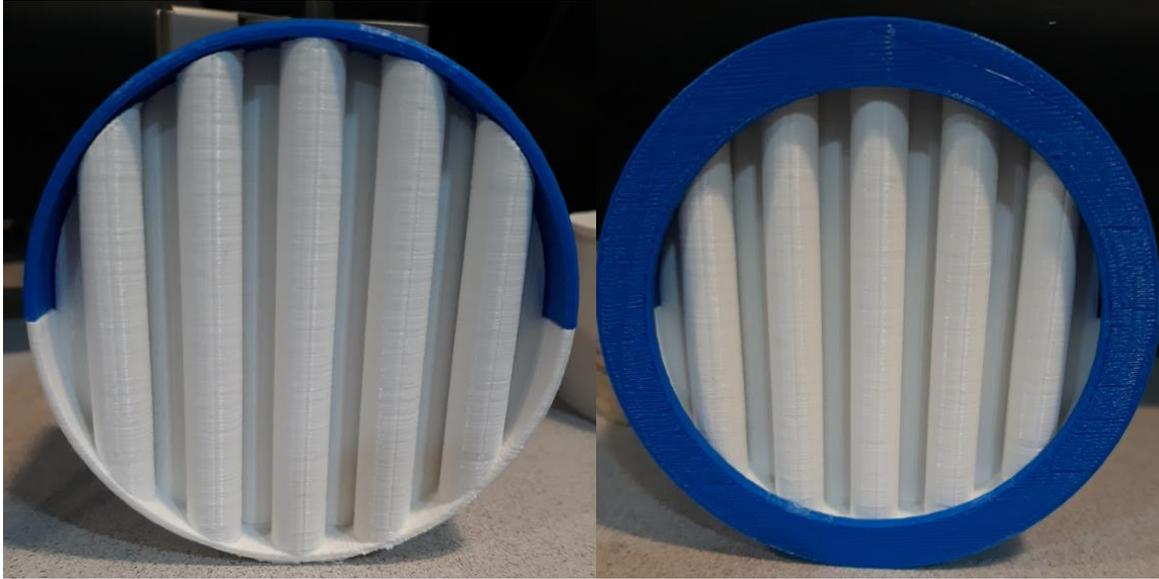
*Figure 2. Printed sample with semicircular cap and complete assembly of sample.*
