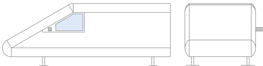
Figure 2: Geometry of the SAE body, used in the research of Müller [1]
