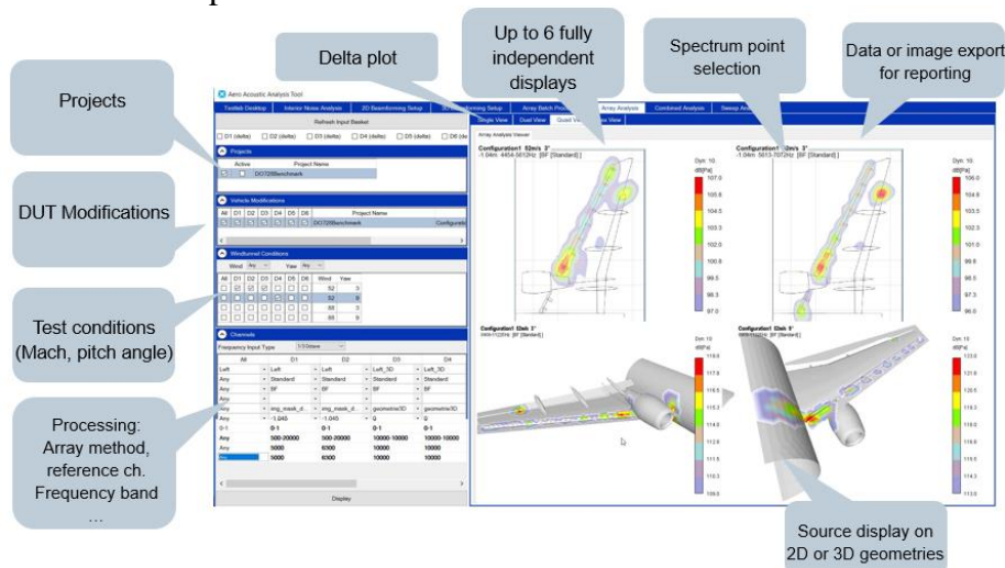
Figure 1 – Data selection view of the aeroacoustic processing software developed for productive wind tunnel testing
