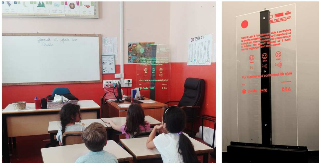
Figure 1. The noise monitoring system with lighting feedback (SEM) located in classroom. Green represents acceptable background noise levels, yellow indicates an increase of them and red means that noise levels are high and annoying.
