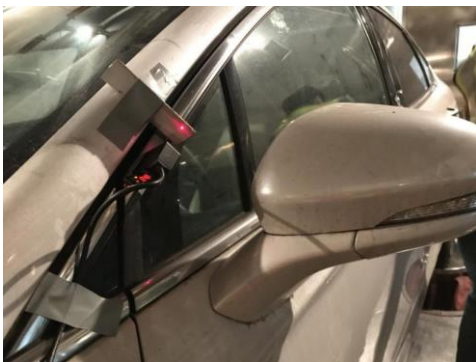
Figure 6 Setup of displacement meter on 4-poster
