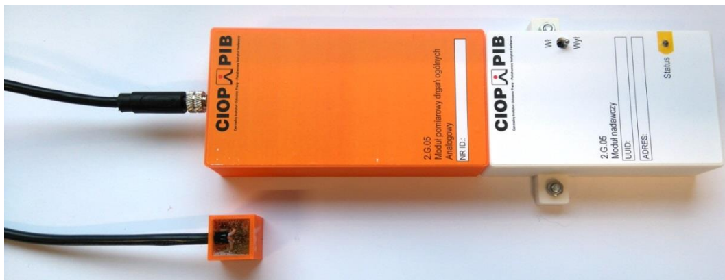
Figure 5. The model of the vibration measuring device.
