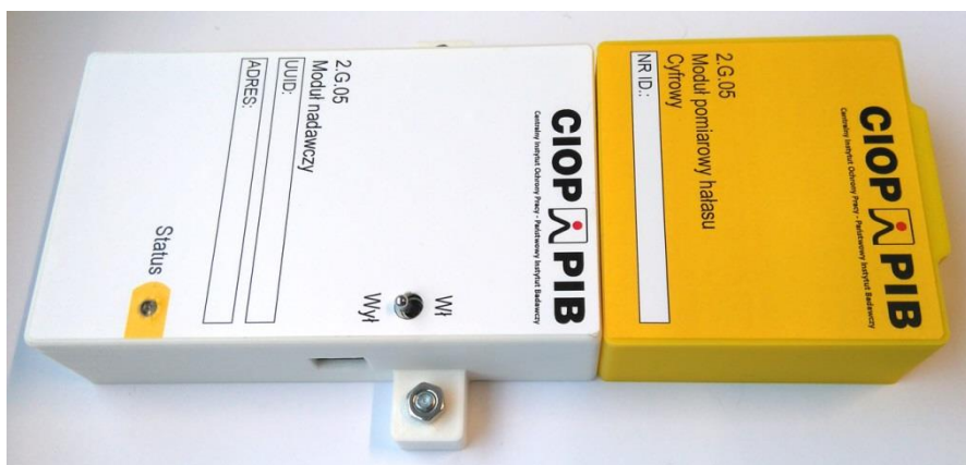
Figure 3. The model of the noise measuring device consisting of communication module (white) and digital noise sensor module (yellow).
