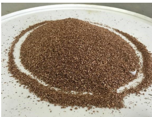
Figure 1: Expanded vermiculite used in the blocks' cavity filling.
