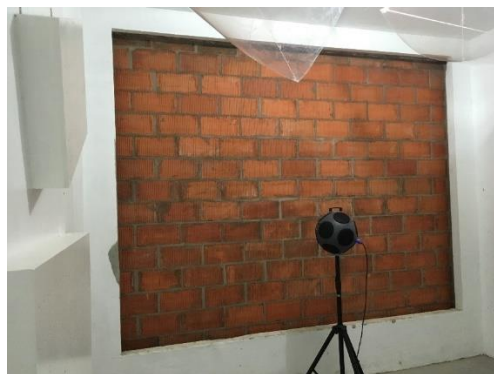
Figure 3: Test specimen in the interior of the chamber for the acoustic tests.
