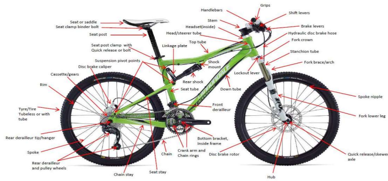
Figure 2.1 - Descriptors of Mountain Bicycle Parts [3]
