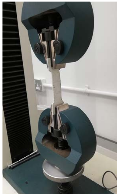
Figure 6: Fibreglass specimen clamped in preparation for determination of modulus of elasticity.
