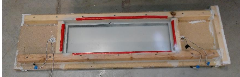
Figure 4. Typical test plate mounting with perimeter support beams
