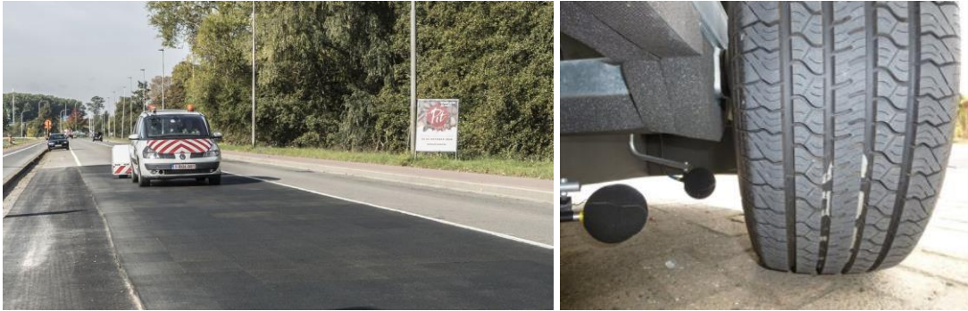
Figure 9 CPX measurements on the PERS test track one day after opening for the traffic
