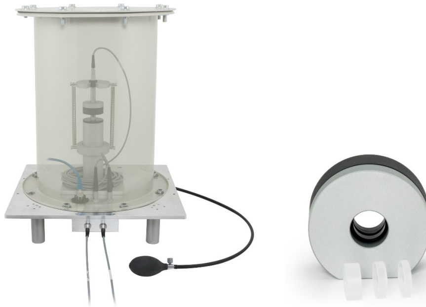
Figure 2: SPEKTRA pressure chamber (left), SPEKTRA coupler holder and three sapphire plane-wave couplers (right)
