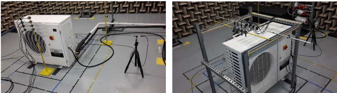
Figure 18: measurement of the outdoor condensing unit in semi-anechoic sound room with free field microphones
