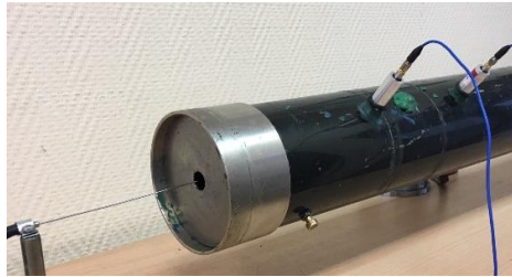
Figure 5. Experimental setup with the Pitot tube fitted to the orifice in the plate.
