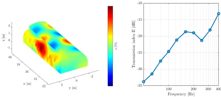
Figure 10: Acoustic pressure fluctuations in the passenger cabin at  $f = 125$  Hz (left) and transmission index (right) for boundary layer excitation
