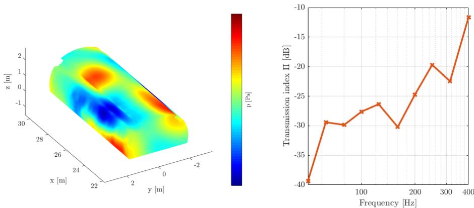
Figure 8: Acoustic pressure fluctuations in the passenger cabin at  $f = 125$  Hz (left) and transmission index (right) for installed jet excitation
