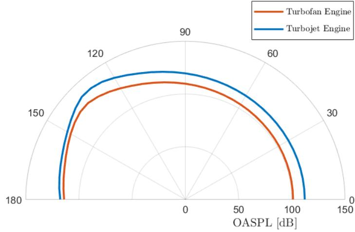
Figure 5: Overall sound pressure level directivity for different engine configurations (distance  $r = 100\text{ m}$ )
