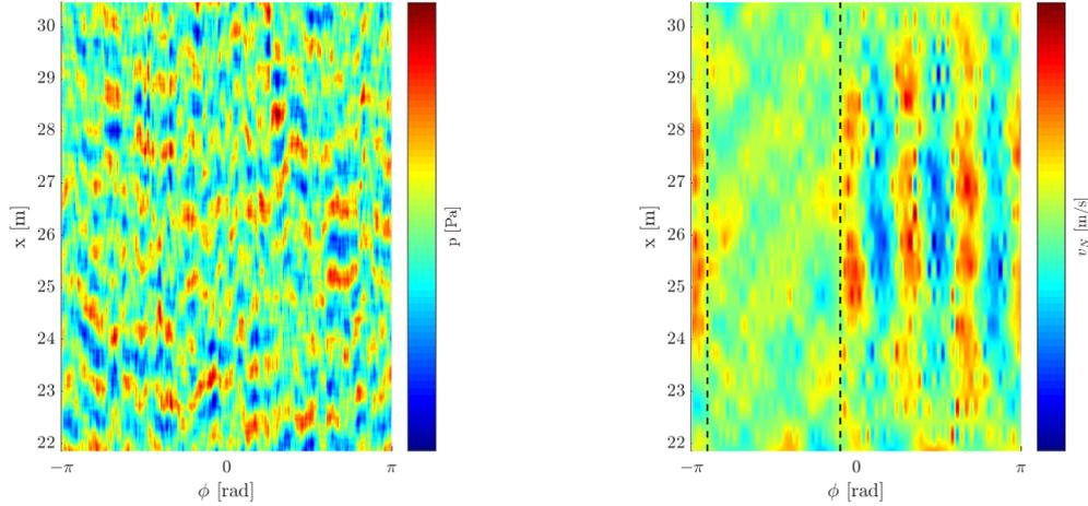
Figure 9: Acoustic pressure excitation (left) and resulting normal structural velocity fluctuations (right) on unfurled fuselage structure at  $f = 125$  Hz due to boundary layer excitation
