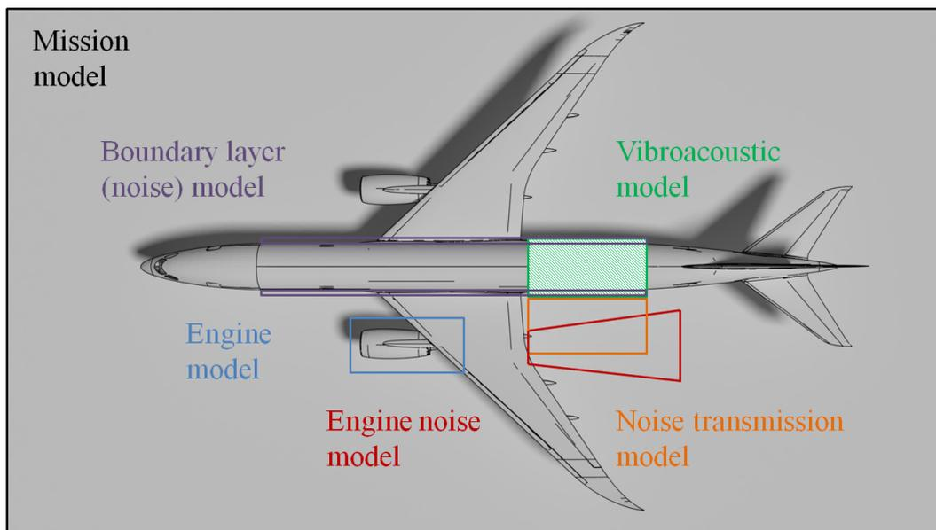
Figure 3: System models of the ACOUSTIC FLIGHT-LAB DEMONSTRATOR
