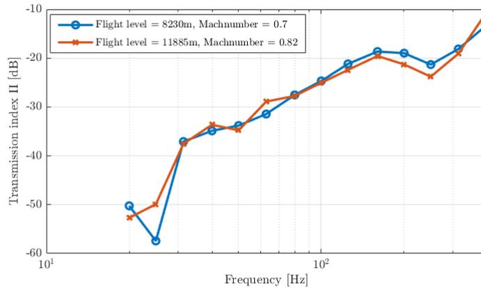
Figure 11: Comparison of transmission index for TBL noise at different mission states
