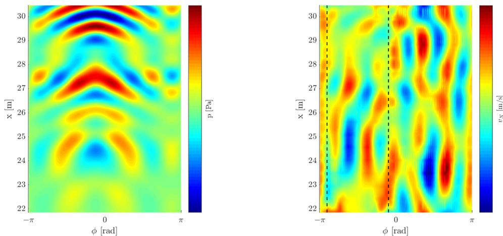
Figure 7: Acoustic pressure excitation (left) and resulting normal structural velocity fluctuations (right) on unfurled fuselage structure at  $f = 125$  Hz due to installed jet excitation
