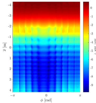
Figure 6: Sound pressure level difference due to shielding of a monopole source (Frequency  $f = 350\text{ Hz}$ )
