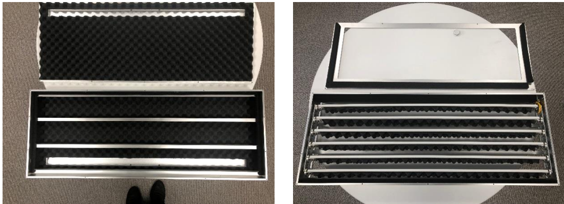
Figure 3. Absorbing material is applied inside the ventilator (Left: Plenum, Right: Louver)
