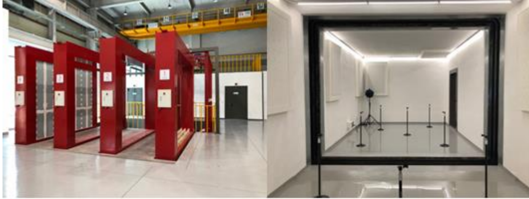
Figure 5. Sound transmission facility (Left: Outside, Right: Inside)
