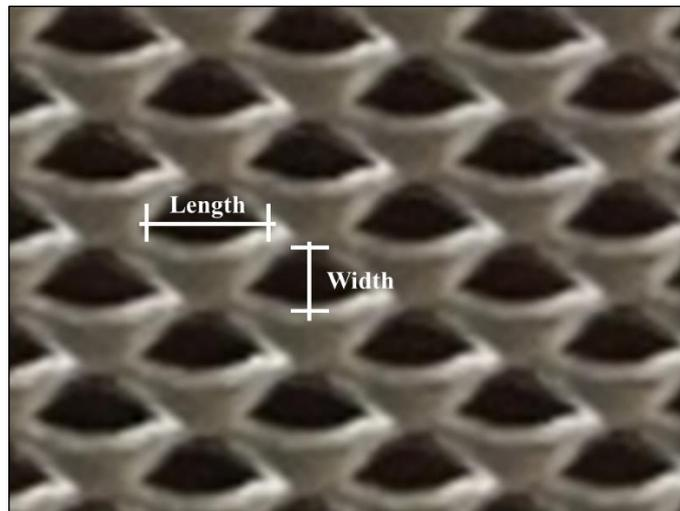
*Fig. 6. Aperture shape of the expanded metal mesh.*
