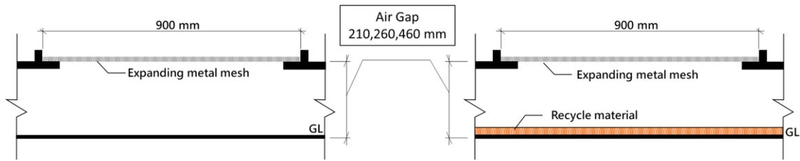
*Fig. 4. Sections of the ceiling systems in the experiments*
