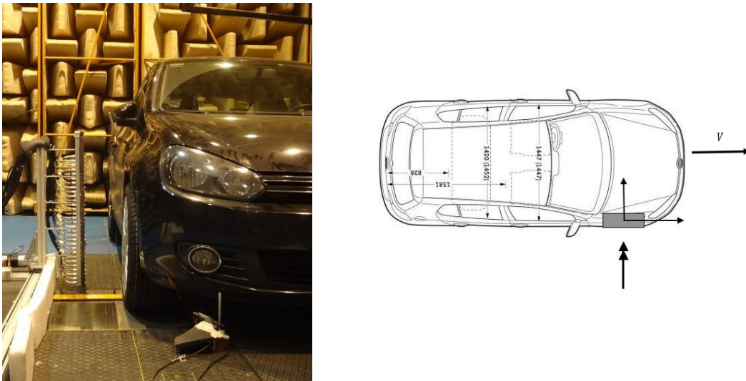
Figure 2. The experimental setup for noise source mapping through the microphone array
