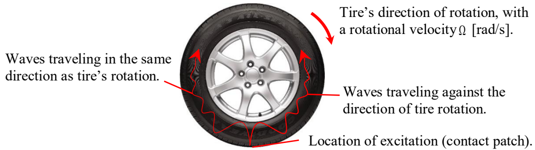
Figure 3. Wave interaction with the rotation of the tire.
