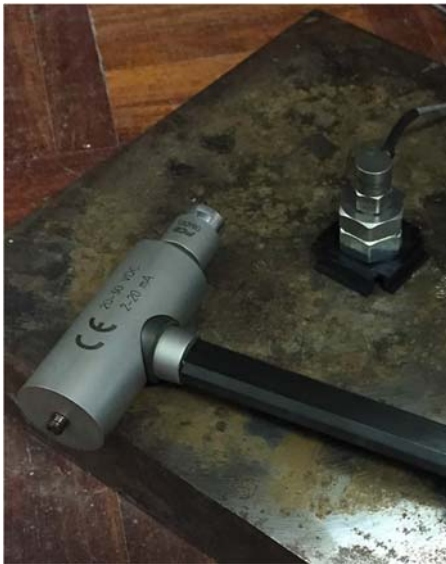
Figure 4 – Modal testing set-up.
