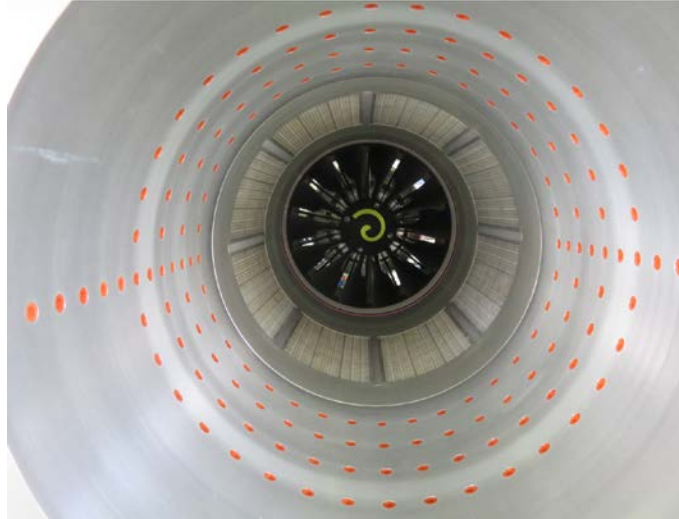
Fig. 5 Acoustic liners and microphone array installed on DGEN fan duct.
