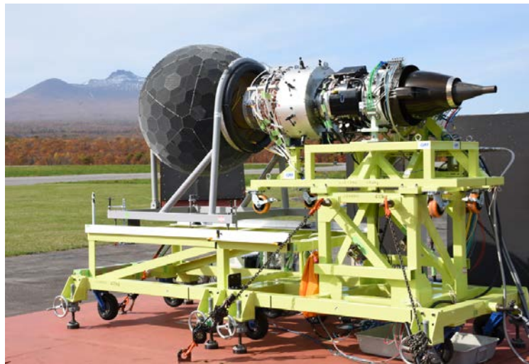
Fig.7 DGEN 380 and inflow control device on the outdoor engine test stand.
