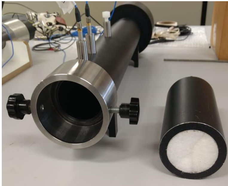
Figure 1: Setup used for the measurement with an impedance tube.
