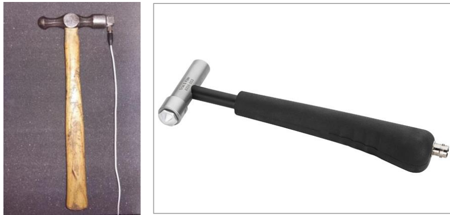
Figure 5 Instrumented tool hammer (left) and a B&K force hammer (right) used in tests
