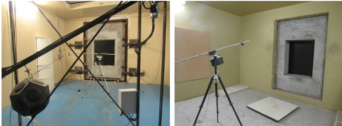
Figure 2 – Transmission Loss facility: source (left) and receiving (right) reverberant chambers.
