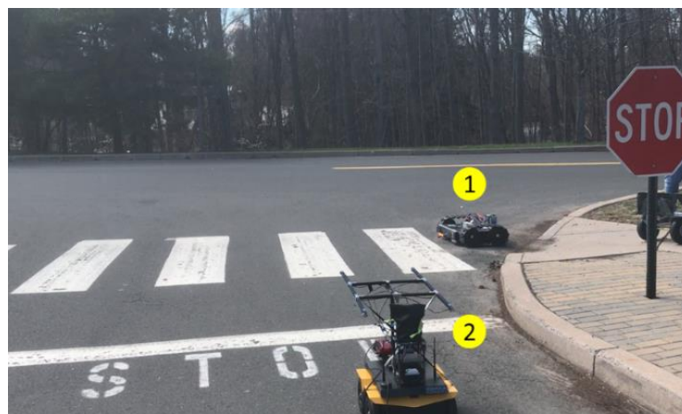
Figure 6. (1) Sound source in motion with a siren, (2) Observer mobile robot.
