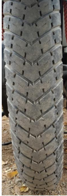
Figure 4: Tread pattern of the two-wheeler tire used in the study
