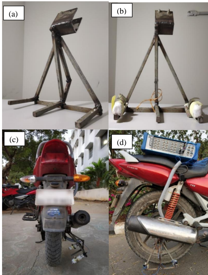
Figure 2: OBSI actual test setup: (a) Fabricated fixture, (b) Microphones mounted on the fixture, (c) Fixture connected to the two-wheeler (rear view), and (d) Longitudinal view
