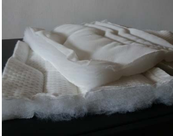
Figure 10 – Acoustical panels from recycled textiles.
