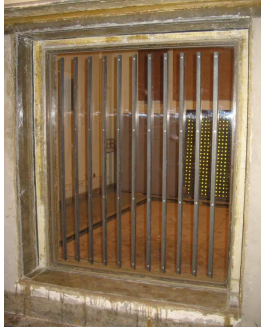
Figure 1: The plate mounted in the small vertical transmission opening of the KU Leuven Acoustics Laboratory.
