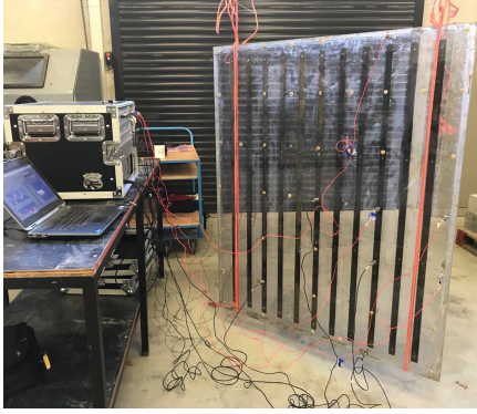
Figure 3: Measurement setup of the dynamic test on the plate with free-free boundary conditions. Figure 4: Mode shapes and natural frequencies of the plate with free-free boundary conditions.
