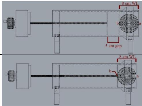
8 cm WL + 5 cm air gap, 1 side closed (a is open b is closed)
