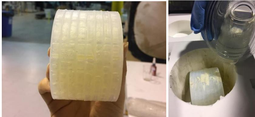
*Fig. 4 Final printout of Web Labyrinth (WL) sample in real size (on the left), while epoxy resin is being cast to the mould to have the final version suitable for Kundt tube measurements. (on the right)*
