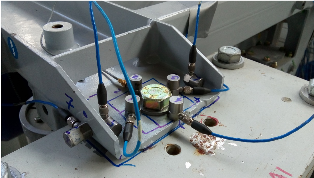
Fig. 4 – Instrumentation of AGTU connection point
