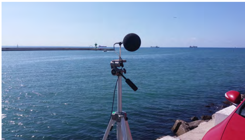
Figure 3: Recording setup at terminal B of Adossat dock.
