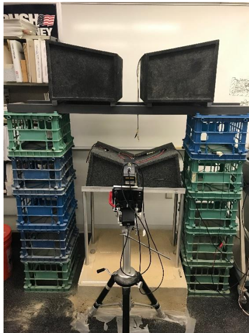
Figure 3: Laser Doppler vibrometer setup with soil box, speakers, amplifiers.
