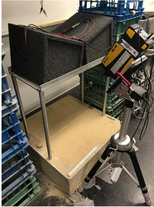
Figure 4: Laser Doppler vibrometer beam on center disc
