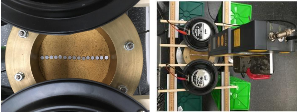
Figure 3. (a) Close-up of the soil plate oscillator SPO with 445 grams of sand loading (density 1.43 g/cc). The upper toroidal brass flange is 5.0 inch I.D., 8.0 inch O.D. and 2.5 inch tall. Reflective 0.6 cm diam disks (1 mm thick) are placed along the sand surface to allow excellent reflection by the Polytec 100 laser Doppler vibrometer. (b) Experimental setup of SPO being driven by airborne sound generated from two 6.5 inch diam, 8 Ω loud speakers. LDV measures the sand particle velocity response vs. frequency at 15 scan locations across the sand surface.
