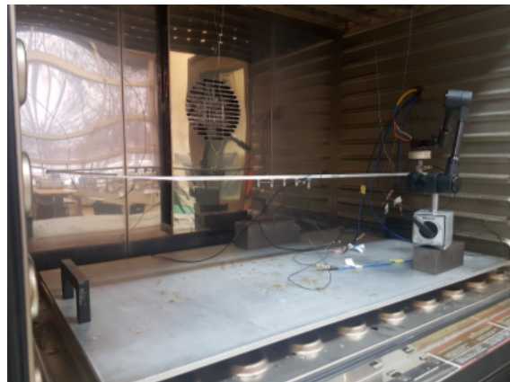
Figure 3: Experimental setup - host beam with ABH and damping layer suspended in the thermal chamber
