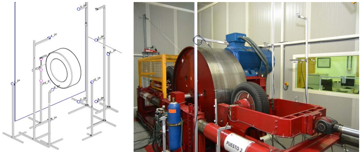
Figure 7. Microphone stands and microphone array around the tyre for an A-DR test.
