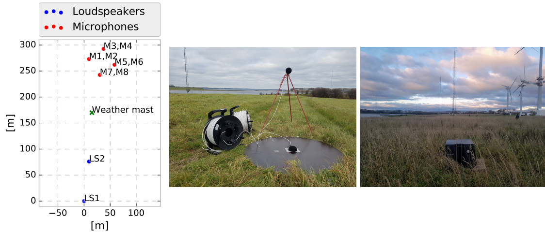
Figure 1: Experimental setup at the Risø campus wind park of the Technical University of Denmark. Left: position of loudspeakers, microphones and weather station. Middle: pair of microphones M3, M4. Right: loudspeaker LS1 and weather mast.
