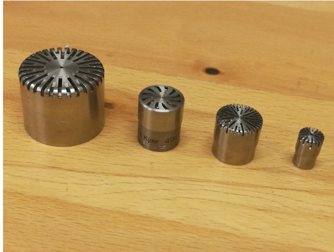
Figure 2: Working standard microphones. On the left a type 1 (WS1). On the center two examples of type 2 (WS2). On the right a type 3 (WS3)
