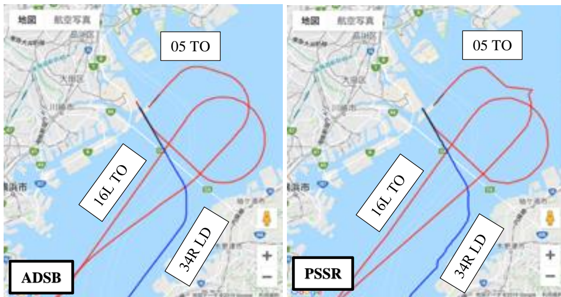
Figure 2 Comparison between ADSB flight path and PSSR flight path
